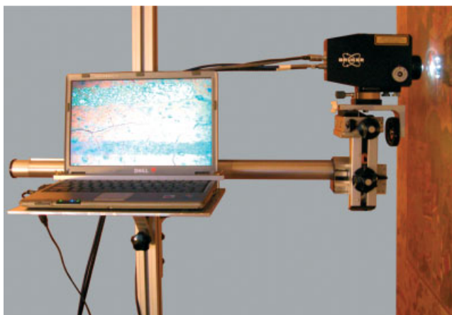
Figure 8. Photograph of the mount of the Raman UNILAB Probe (Bruker Optics) in front of the thangka ET10 of Fig. 9. A Manfrotto tripod on wheels (not visible) was vertically extended by a 40 × 40 mm Kanya rail. It holds a horizontal arm, taken from the Sinar large-format camera module system, that carries a Sinar P Front Standard allowing the UNILAB Probe to be moved in a controlled manner in all directions. The video image of the area sampled by a 10× objective is displayed on a Dell X1 computer screen.
