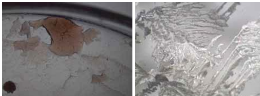
Figure 17: examples of solidified oil and dendritic solidification
