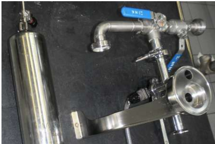
Figure 1 : Installation de filtration Millipore®
