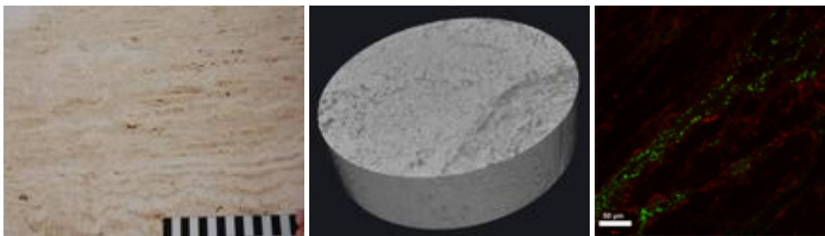
Fig. 1. Left: Field image of layered pond facies in Cakmak (Denizli Basin, Turkey). Centre: Reconstructed \mu -CT image of proximal slope plug (2.5 cm diameter, resolution 11.7 \mu\text{m}^3 , Turkey). Right: Confocal laser microscopy image of thin section from pond facies (Cakmak, Turkey). The thin section was selectively stained for DNA (red) and plasma membrane (green).
